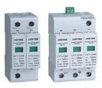
LY1-(C)7 series surge protective device is suitable for the new energy wind/solar power generation system ,its working voltage covers 500V,800V,1000V.lt is installed in the main power system at DC circuit,to protect against the indirect lightning current, direct lightning current or other instantaneous over voltage.
