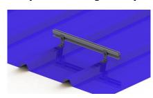
When we installed L-foot, and we can fix the rail at any side of L-foot kit according to the actual condition
