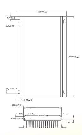
DM260/DM300 dimensions: Overall dimensions: 200\*122.5\*56mm Mounting dimensions: 175\*113mm Mounting hole diameter: φ3.5mm
