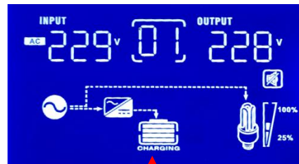
Mains mode (battery capacity icon flashing when charging, when no charging or complete it will stop flashing )
