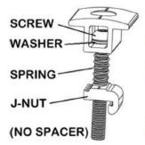
\*\*Make sure the SPACER is removed\*\*
