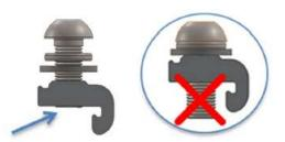
Bottom of screw is flush with J-Nut
