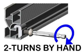
STEP-3: Once the piece is aligned and ready to tighten, use an electric drill, fitted with the Lock Solar security drill tec bit (#110-001) and tighten to 8Nm of screw torque.
