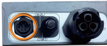
Communication connector of inverter
